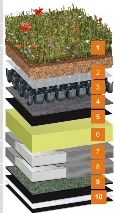
Build-up to achieve 0.16 on a concrete deck
