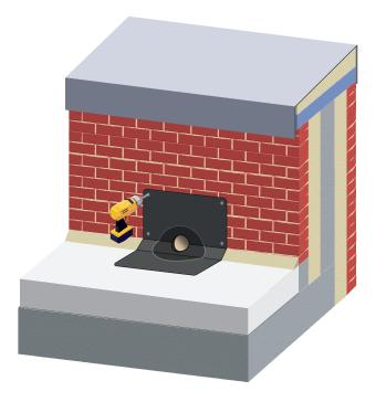
**3:** Apply the waterproof layers, bonding the underlayer on to the bituminous connection flange provided.
