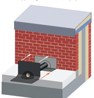
2: Mechanically fix the flange of the outlet body to the wall.
