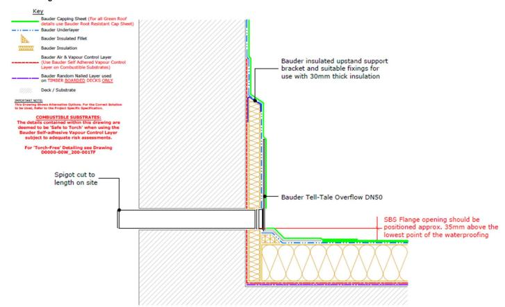
Installation Guidance and data: Please refer to the Bauder Installation Guide and project specification for guidance.
