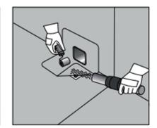
The metal base plate of the outlet must be mechanically fixed to the structural deck.
