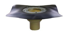
The thermal value of the rigid foam body prevents condensation from forming on the underside of the outlet body. The integrated screw down clamping ring ensures security between the waterproofing system and the outlet.
