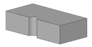
For concrete decks, the roof outlet hole ( $\varnothing$  250 mm) should be pre-cast in-situ so the outlet can be installed by the roofing contractor when the waterproofing system is installed
