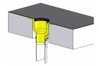
9. Place the clamping ring into position ensuring it provides a physical clamp between the Bauder Protection Sheet and outlet body. Tighten the countersunk head screws supplied with a screwdriver.
