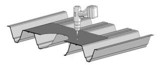
In the case of profiled galvanised steel decking, the edges of the cut hole to be treated to prevent future corrosion.
